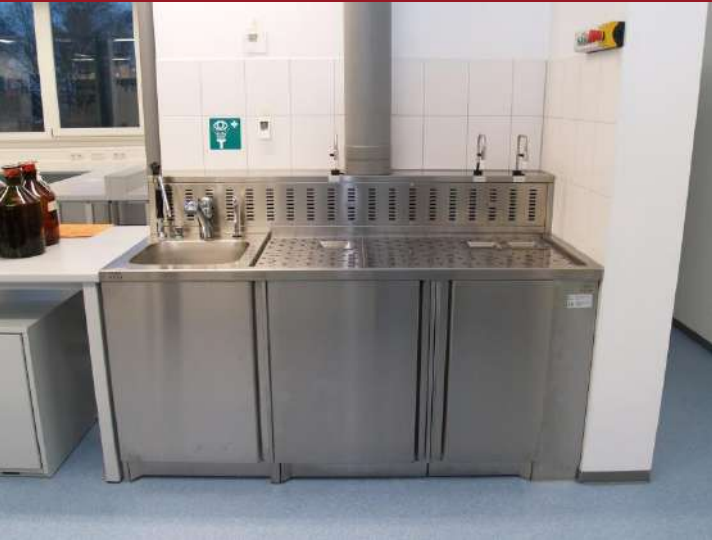
Dispensing system for formalin, xylol and ethanol with vacuum system downwards and backwards throughout the perforated sheets
