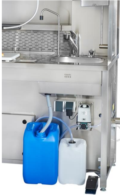
Formalin waste drain with connection to blue 20 liters tank (left) for used formalin At the right side: white 10 liters tank with connection adapter for formalin pump
