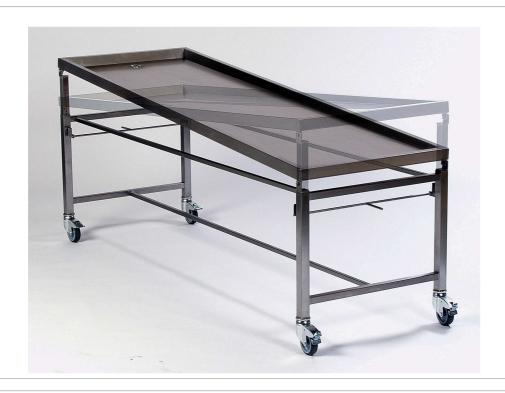
The table is completely made of stainless steel (Material no. 1.4301 – ANSI 304). The table top features a high surrounding border and a negative inclination arranged diagonally to the drain. The substructure consists of rugged, torsion-resistant stainless steel profiles with 4 steerable wheels with break and special roller bearings, permanently lubricated and maintenance-free. The table top is manually height-adjustable on both sides from 750 to 950 mm and can be fixed every 20 mm.
