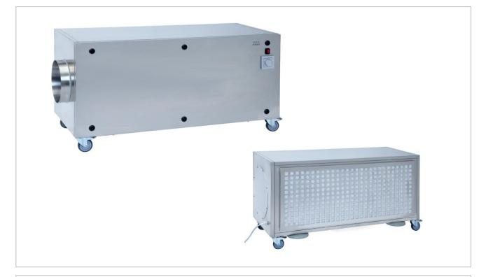
Suitable for down-draft grossing tables, consisting of: Solid stainless steel housing with 4 controllable and lockable wheels, access panel at the up front for easy access to all filters and the exhaust air fan and backside with exhaust air grid and filter fleece.
