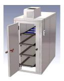
Morgue refrigeration unit KZM 40/450 To storage 4 body trays in 4 levels 1 Door 680 x 2000 mm Made of 80 mm CFC –free polyurethane rigid Foam, coated outside steel Dimensions W/D/H: 1210 x 2260 x 2260
