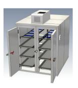
Morgue refrigeration unit KZM 40/850 To storage 8 body trays in 4 levels 2 Doors 680 x 2000 mm Made of 80 mm CFC –free polyurethane rigid Foam, coated outside steel Dimensions W/D/H: 1910 x 2260 x 2260 Article No.: 040.020.020
