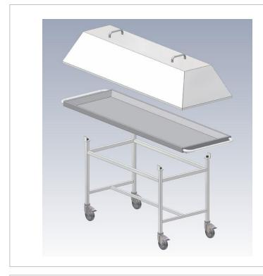
The Transport Truck TW 52/050 has a rugged, torsion-resistant frame structure of stainless steel profiles. 4 solid rubber wheels, 2 of them lockable, diameter 125 mm with special roller bearings, permanently lubricated and maintenance-free, ensure an absolutely noiseless movement. The top of the transport truck is furnished with 4 rubber pads to include a body tray.
