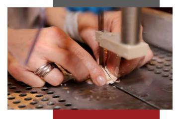
This stationary cutting-grinding system with a fixed large work table is specially designed for preparing tissue, bone and composite materials for histological evaluation and is therefore restricted exclusively for this use.
