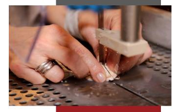
This stationary cut-off machine with fixed work table is specially designed for preparing tissue, bone and composite materials for histological evaluation and is therefore restricted exclusively for this use. A diamond-coated, high-precision cutting belt is used for cutting. The device works according to the principle of cut-thin grinding.
