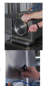
The adjustment device on the impeller makes it quick and easy to correct changes in the bandsaw blade rotation.
